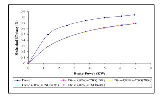
Fig.3. Brake power(kW) Vs Mechanical effi.(%)
