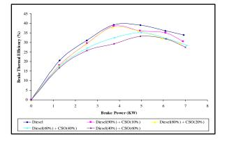
Fig.4. Brake power (kW) Vs Brake thermal efficiency(%)
