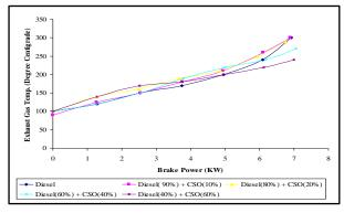
Fig.5. Brake power (kW) Vs Exhaust gas temperature (  $^\circ\mathrm{C}$  ).
