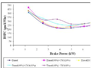
Fig.2. Brake power(kW) Vs BSFC(gm/kWhr)
